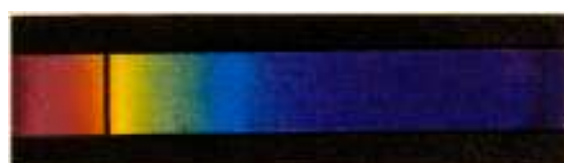
Spectrum showing the absorptive power of Iodine vapour (Fig 34)
